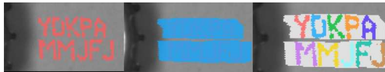
The process of splitting text into lines using region morphology filters.
