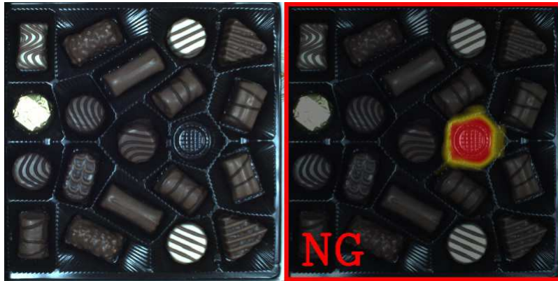
An example of a missing object detection using DL_DetectAnomalies2 tool. Left: The original image with a missing element. Right: The classification result with a heatmap of anomalies.
