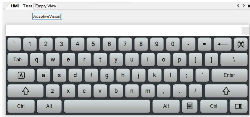
The example of using VirtualKeyboard for entering data on HMI panel into TextBox control.
