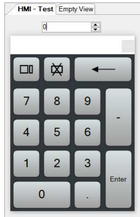
The example of using VirtualKeyboard for entering data on HMI panel into NumericUpDown control.
