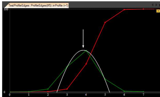
Fitting a parabola to three consecutive points.
