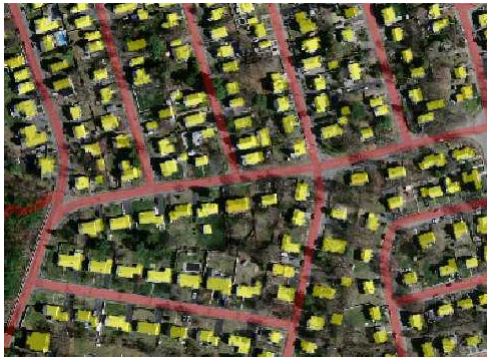
An example of marking two different classes (red roads and yellow buildings) in the one image.
