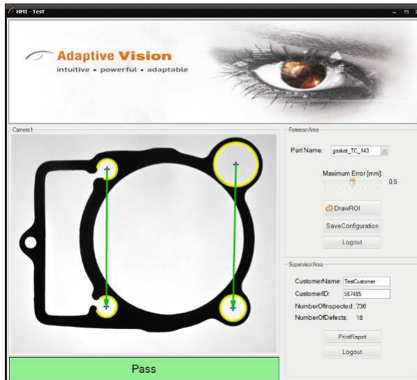
HMI with Unlocked ForemanArea and SupervisorArea.
