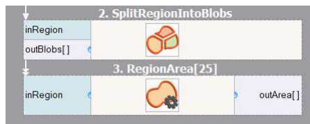
An array connection.
