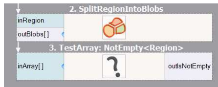
The TestArrayNotEmpty filter used to verify if there is at least one blob.
